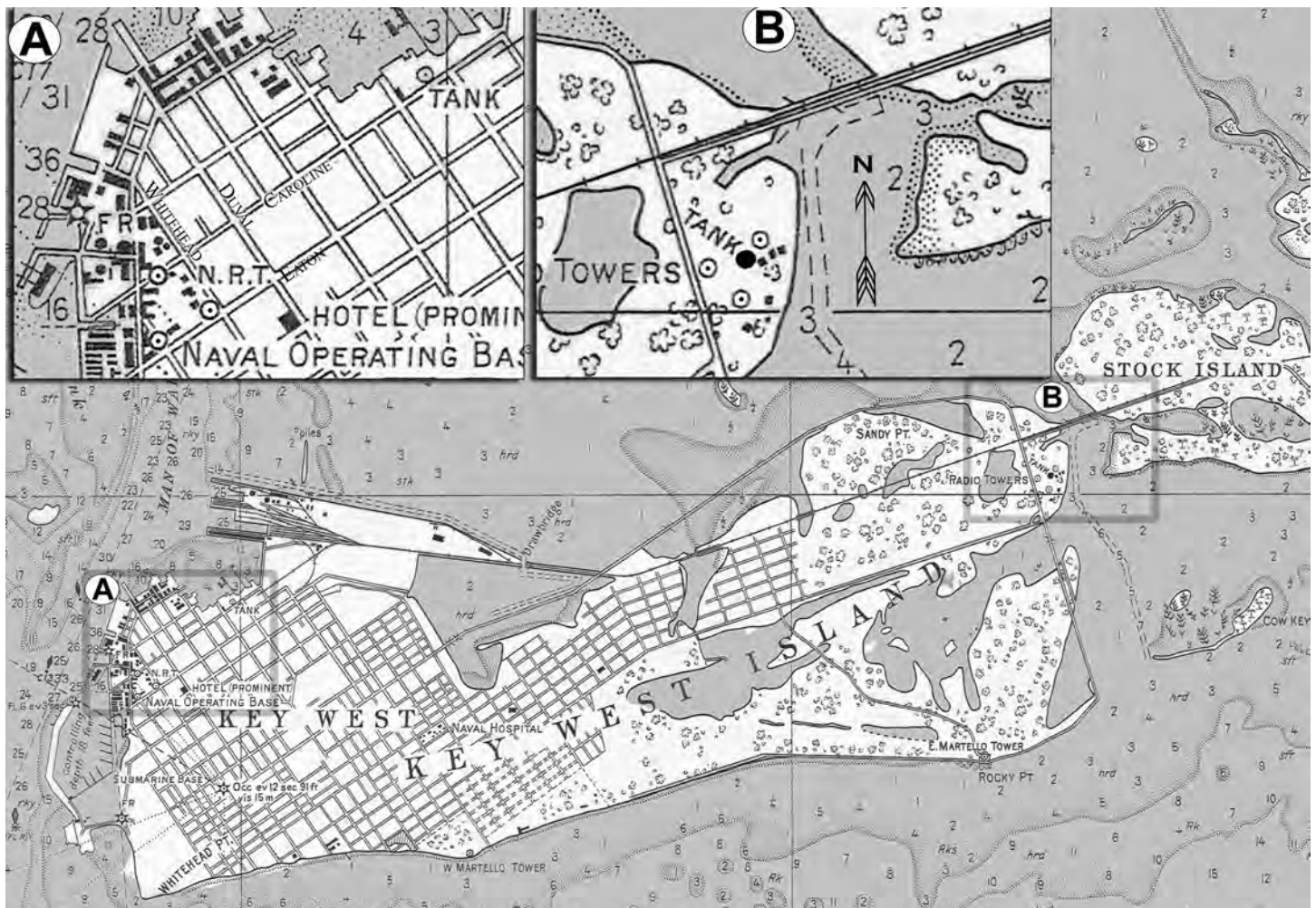
After 1914, the Navy’s wireless facilities in Key West were comprised of two stations; the transmitter station was located on the west end of the island in the Navy Yard (Inset A--the towers are indicated by a white circle with a dot in the middle) while the receiving station was located on the east end of the island (Inset B) in a relatively undeveloped area. This arrangement helped isolate the sensitive receivers from interference from static generated by local industrial activities. The chart above was issued in 1932 after the boulevard was constructed. Photo credit: The Author.
